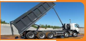
•The basket of damper truck in movement remains at the raised position
